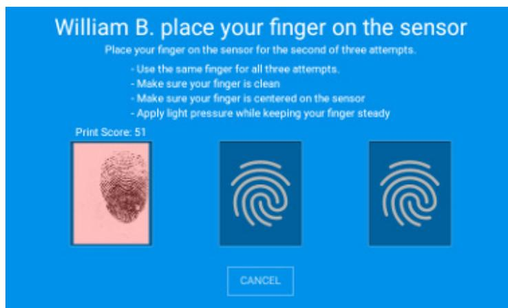
Once three scans are completed and the employee has at least one scan of 65 or higher, the clock stores the landmarks from the highest scored fingerprint.
