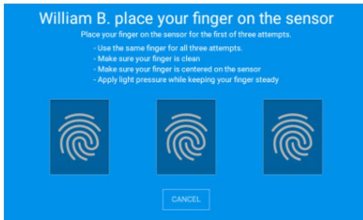
After each scan, the clock beeps and the employee should remove their finger from the sensor and repeat, as instructed by the clock. The screen also displays an image of the fingerprint with a score indicating the quality of the scan. The clock needs at least one scan with a score of 65 or higher.
